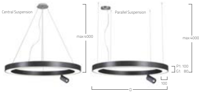
Minimal suspension height for the central suspension
