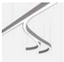
LIQUID LINE Y-JUNCTIONS SUSPENDED | G3/P3 234
